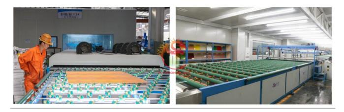
**Reason 3:** Our tempered glass production line, each worker craftsman has up to 8-10 years of fabricate experience, while the production supervisor has up to 15 years of experience. We strive to match the appropriate heating temperature and pressure in order to prevent damage to patterns of ceramic fritted glass tabletop, making our ESG glass more durable with low self-explosion rate of 0.1-0.3%, thus avoiding many safety issues for customers during use.
