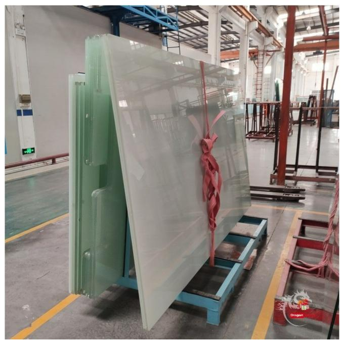
Heat Strengthened Glass has been gaining increasing traction as an innovative material for use in the construction industry. The process of heat strengthening is a specialized version of the more common tempering technique and can produce glass with superior strength and a higher level of break resistance than normal float or annealed glass.
