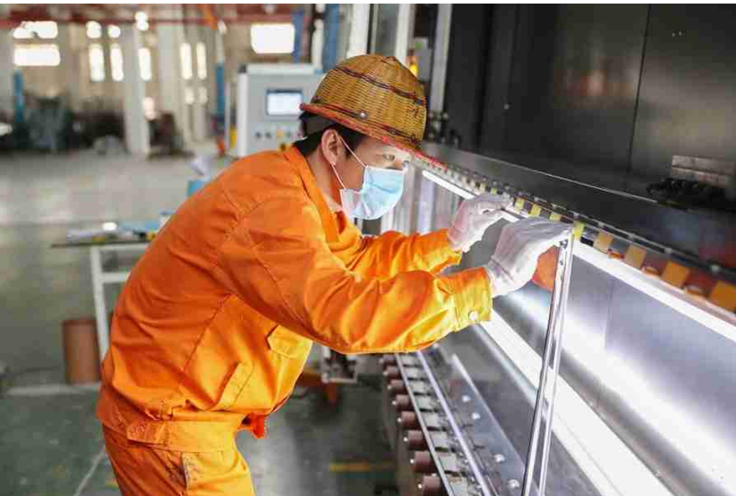
Carefully matching the butyl & aluminum spacer with the glass
