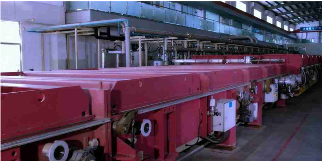
Large area sputtering line for reflective glass production.
