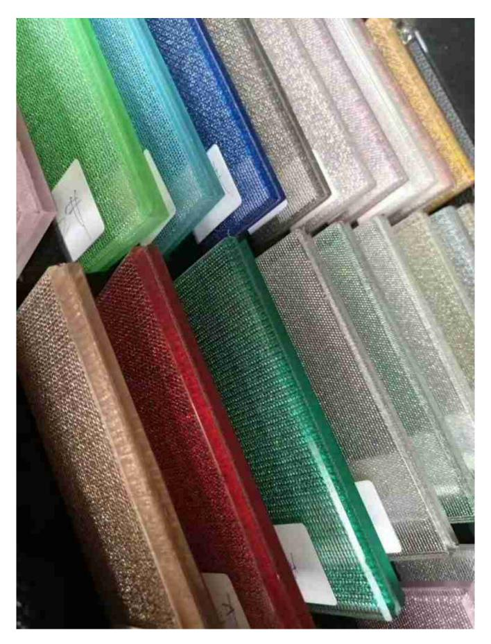
Fiber laminated glass is made of two or three layers of glass with PVB or SGP or EVA in the glass between, to process with high temperature and high pressure.
