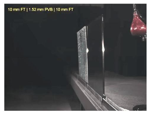
This is a helpful video to show you the difference of SGP laminated glass vs pvb laminated glass vs tempered glass.
