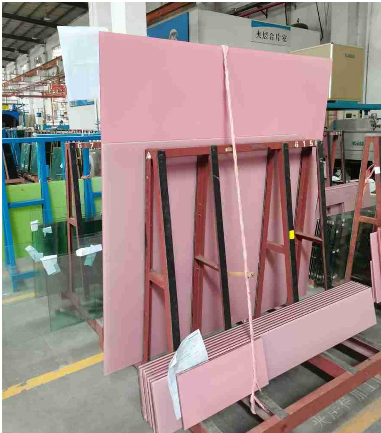
Pink laminated glass is using one or two pieces of pink ceramic fritted glass permanently bonded together with [PVB interlayer](#) by high temperature and high pressure.
