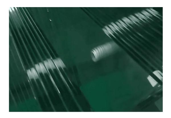
Laminated glass is made with two or more panes of glass that are held in place with the help of an interlayer to form a permanent and strong bond. The interlayer is typically made of Polyvinyl Butyral (PVB). The PVB interlayer bonds with both the layers of the glass and hold it together to form one strong, intact uniformed layer upon a harsh impact. This bond between the PVB sheet and the glass is a chemical bond and thus it does not shatter easily.
