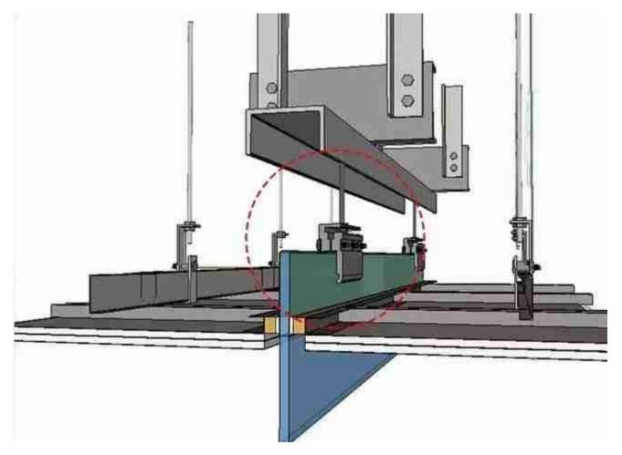
6. After all the glass partitions are installed, inject the colloid. When injecting the colloid, we need to divide it up, down, left, and right. We need to operate from the top and bottom, then from the left and right, and then scrape it all at once.
