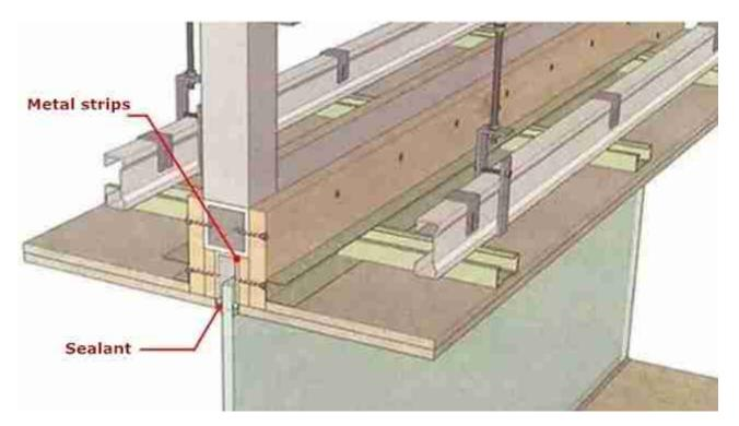
3. Install the steel components at the bottom of the channel according to the size requirements of the drawings. After installation, use expansion bolts to fix and install the steel glass tank on the upper part and on both sides. Then, check the installed glass tank to ensure that it is straight and fix it.
