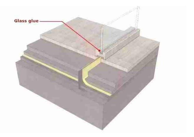
5.Install the glass partition, before install, clean the glass slot to ensure the cleanliness of the surface, so that can install it inside! Afterward, adjust the glass wall partition to ensure it is fixed.
