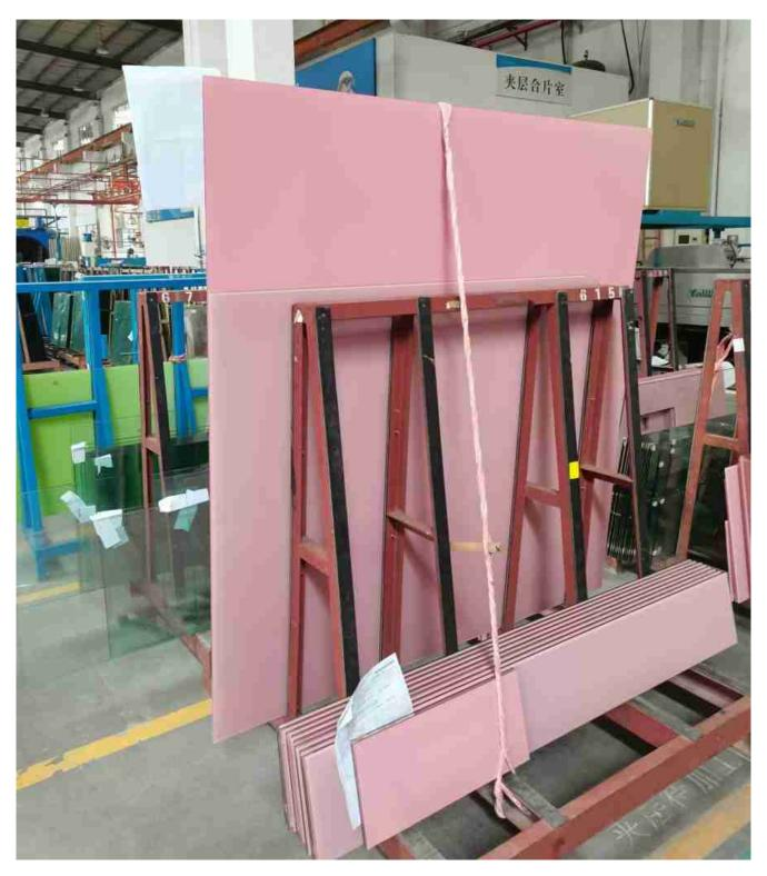
Pink laminated glass is using one or two pieces of pink ceramic fritted glass permanently bonded together with <a href="PVB">PVB</a> <a href="interlayer">interlayer</a> by high temperature and high pressure.
