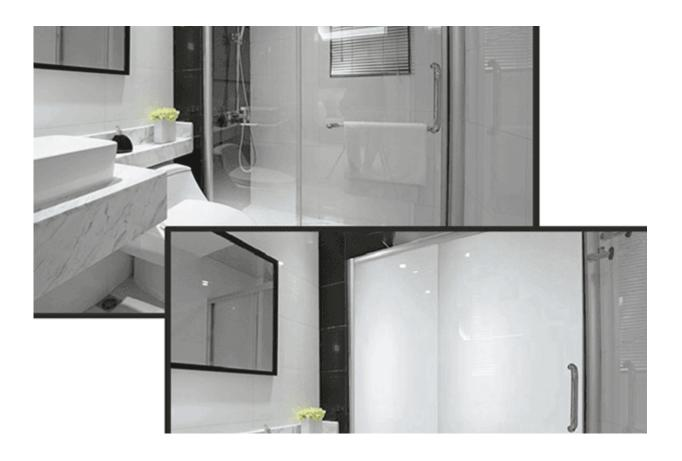
PDLC (Polymer Dispersed Liquid Crystal) is a light modulating material comprised of droplets of liquid crystal uniformly dispersed in a transparency or translucency, flexible plastic film. When power off, coming visible light scatters through the PDLC, and the film turns translucent; When power on, coming visible light transmits the PDLC and the Film turns clear.
