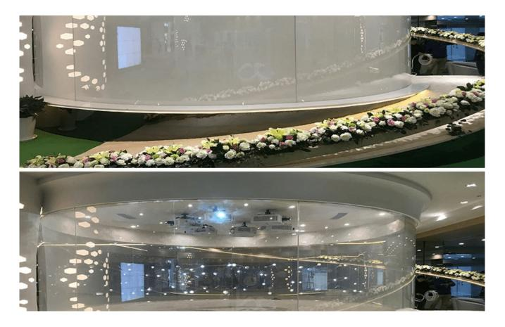
PDLC stands for polymer-dispersed liquid crystals which can be engineered into end-products such as smart windows, office partition, smart glass displays and smart consumer electronics, giving privacy, security and energy efficiency. How does PDLC smart glass work?
