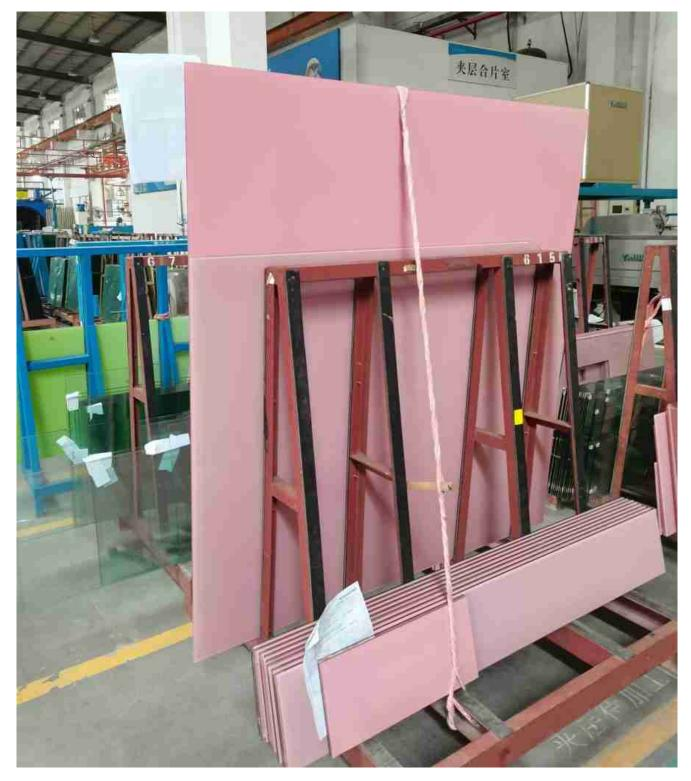
Pink laminated glass is using one or two pieces of pink ceramic fritted glass permanently bonded together with <a href="PVB">PVB</a> <a href="interlayer">interlayer</a> by high temperature and high pressure.
