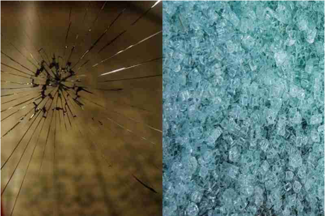
herdet glassbrudd vs float glass brudd
