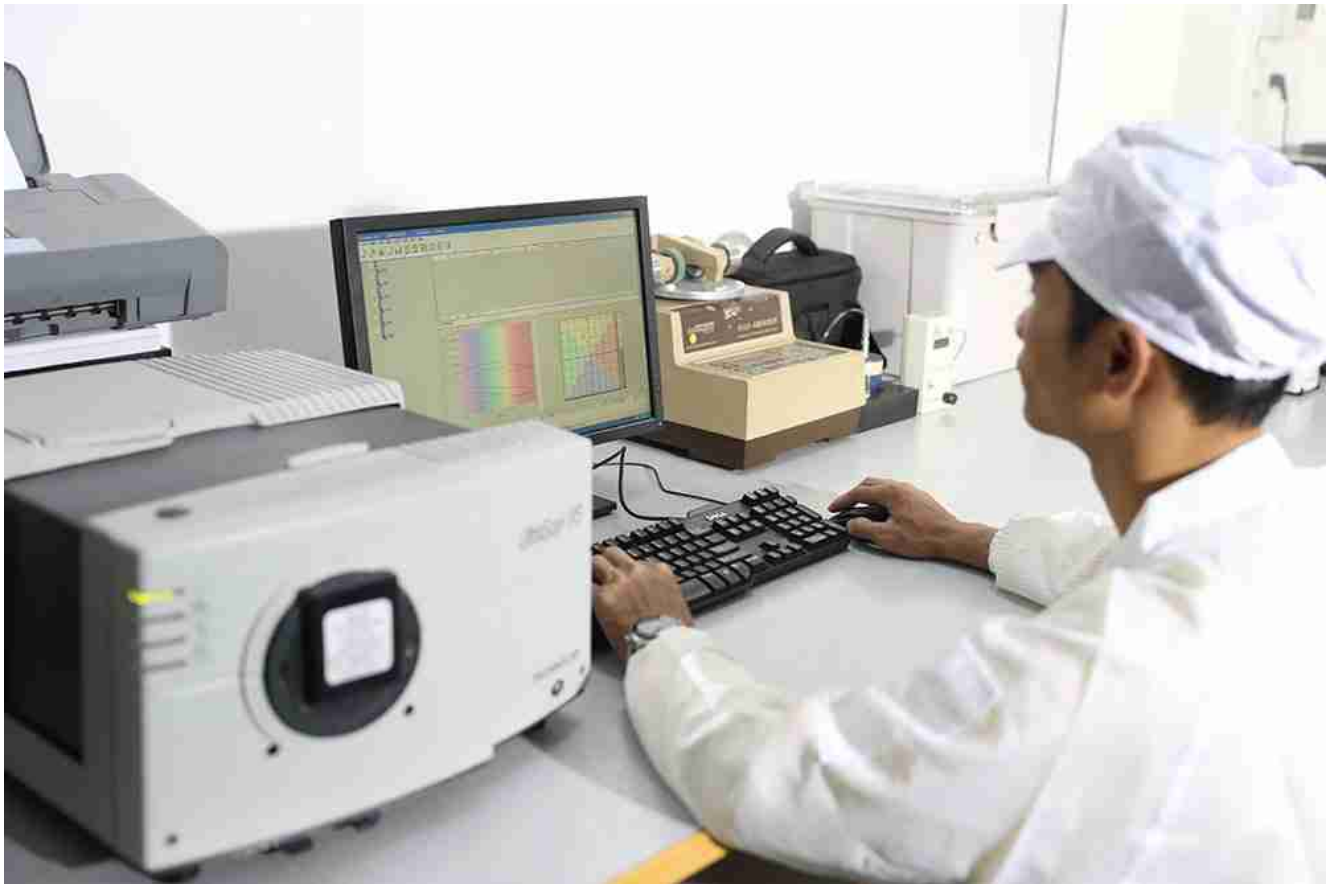
SDG energy saving glass ltd color uniformity inspection
