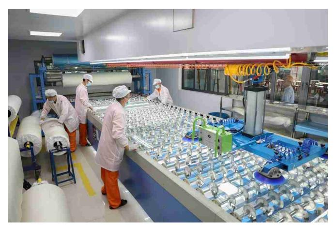
The production of wet laminated glass and EVA laminated glass should be grouted/combined in a clean environment to avoid contamination of the glue/EVA film during the grouting/combination process.
