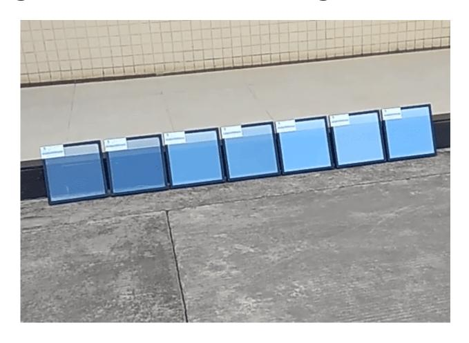
Low-E, or low-emissivity, glass was created to minimize the amount of infrared and ultraviolet light that comes through your glass, without minimizing the amount of light that enters your home. Low-E glass windows have a microscopically thin coating that is transparent and reflects heat. The coating is even thinner than human hair! The Low-E coatings keep the temperature in your home consistent by reflecting the interior temperatures back inside.
