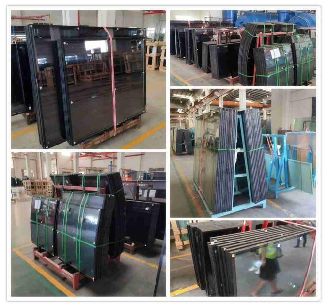
Argon Gas filled double glazing glass, curved shape, and flat shape.
