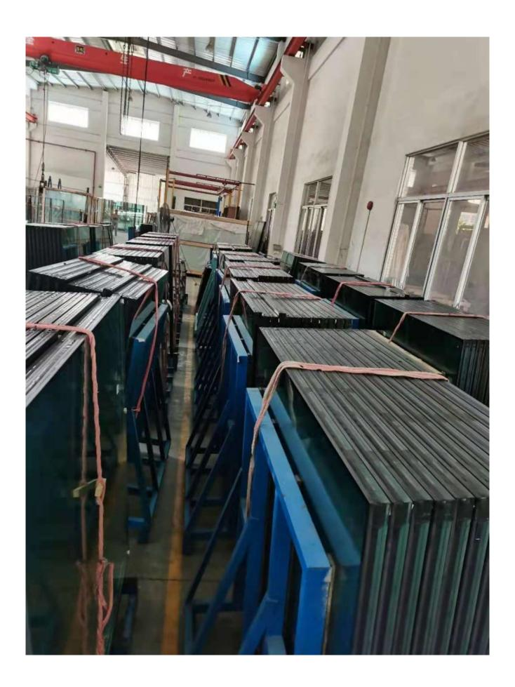
**laminated IGU glass** is also called laminated insulated glass, which is a combination of insulated glass and laminated glass, and is commonly used in curtain walls and sunrooms.
