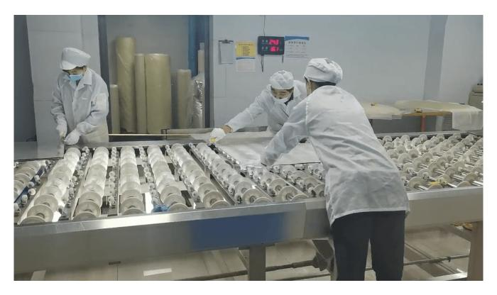
Laminated tempered glass is using two or more pieces of tempered glass panels sandwich with interlayer material like PVB or SGP or EVA material, enduring high pressure and high temperature, thus making the joint of glass permanently together. When one or more panels in the laminated glass are broken due to extreme impact, the broken pieces will still glue together with the PVB or SGP interlayers. Preventing glass pieces from spreading and ensure safety.
