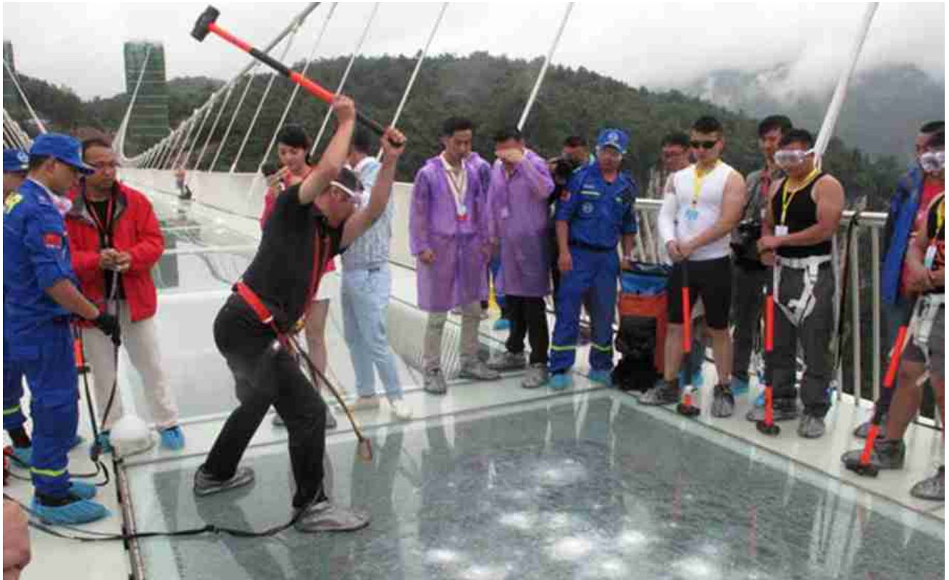
SGP laminated glass flooring enduring strong impact testing
