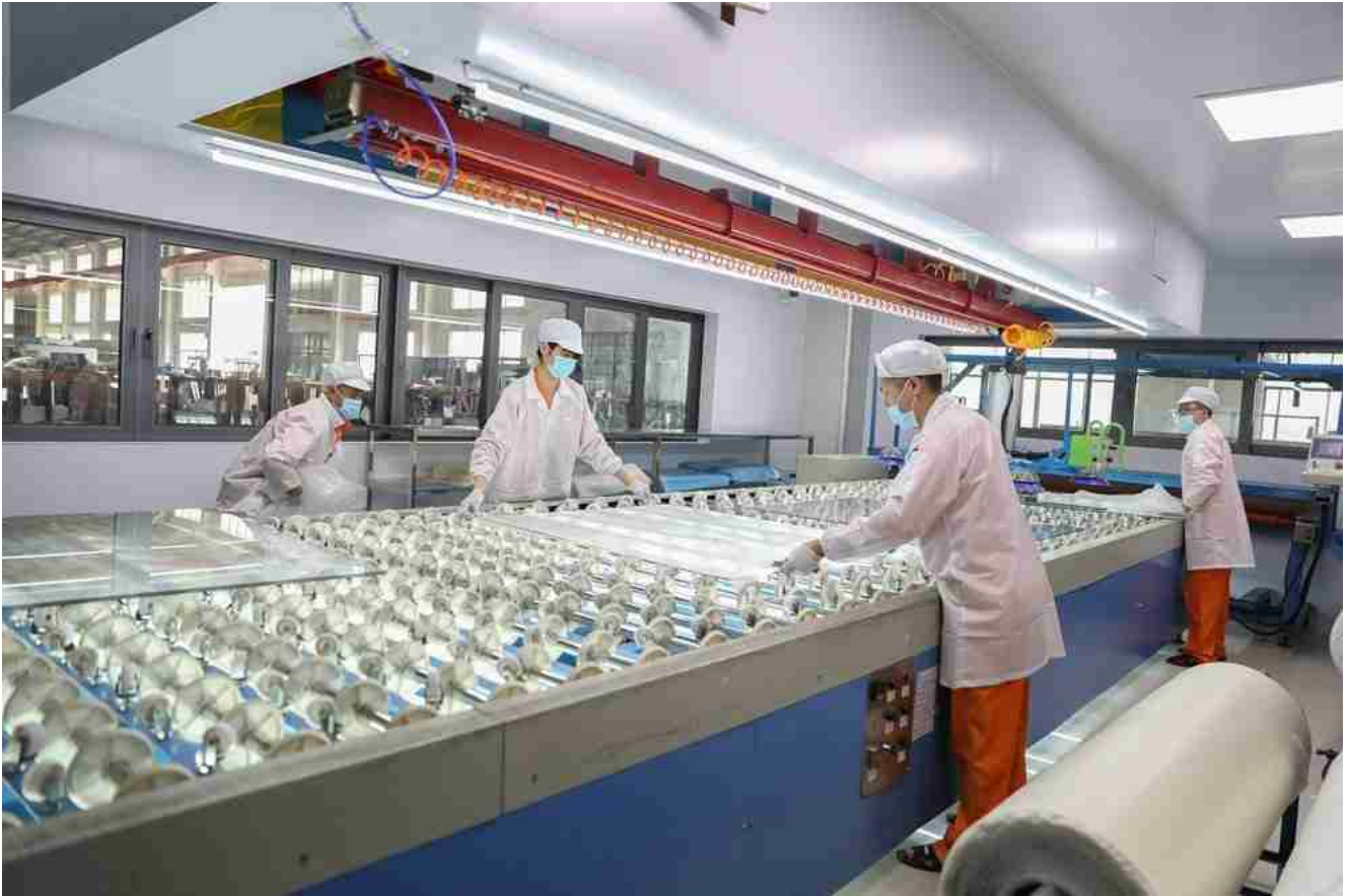
Lamination process in a dust free room
