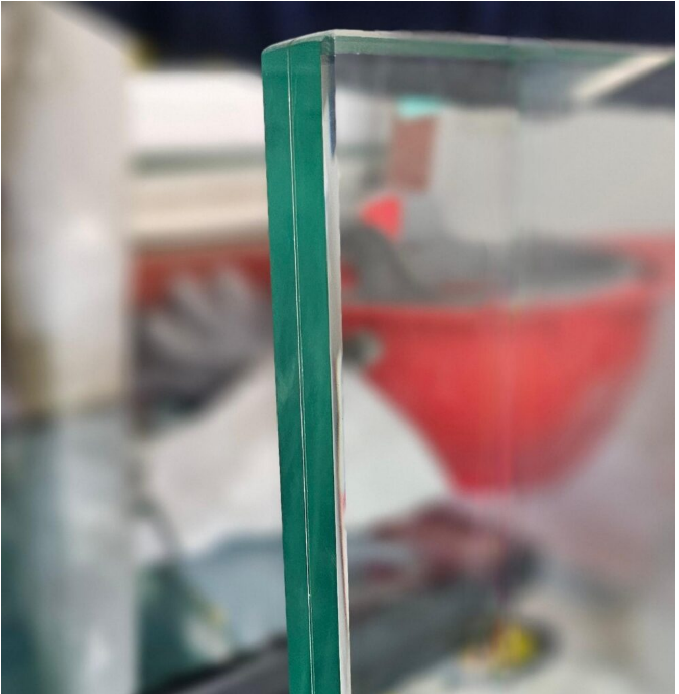
Integral Edge of 20mm Safety Laminated Glass
