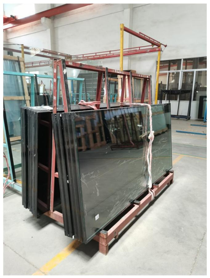
Strong plywood crate packing to avoid the damage of <u>insulated</u> <u>glass</u> during long-distance transportation.
