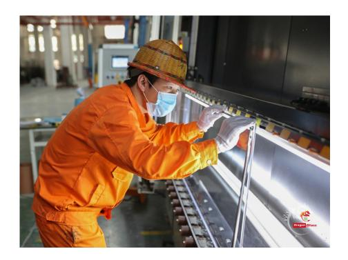
Two pieces of tempered glass are separated by one 16A-27A aluminum spacer and sealed together at the edge, and aluminum shutters built inside, the insulating airspace is filled with dry air or Argon inside to slow the heat exchange and reduce noise levels. The aluminum spacer is filled with silica desiccant pellets to ensure the removal of any moisture in the airspace.
