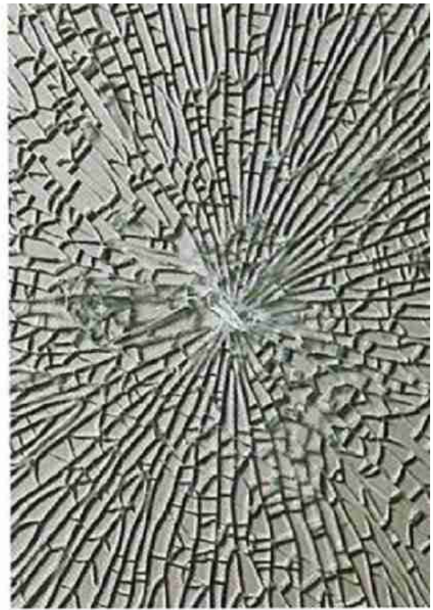
Breakage pattern – Tempered Glass
