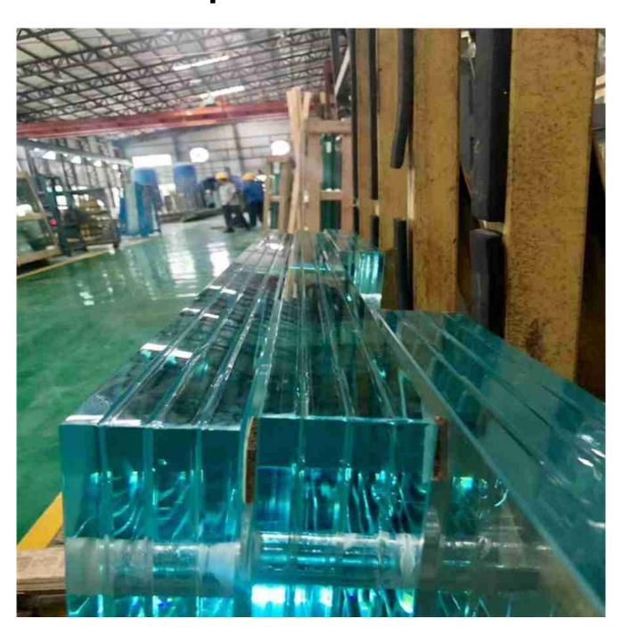
Laminated tempered glass is using two or more pieces of tempered glass panels sandwich with interlayer material like PVB or SGP or EVA material, enduring high pressure and high temperature, thus making the joint of glass permanently together. When one or more panels in the laminated glass are broken due to extreme impact, the broken pieces will still glue together with the PVB or SGP interlayers.
