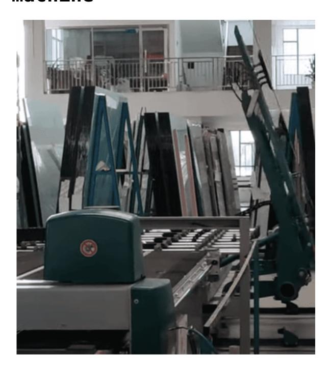
Auto cutting machine, this machine ensures the glass cutting smooth, with accurate dimensions and good quality.
