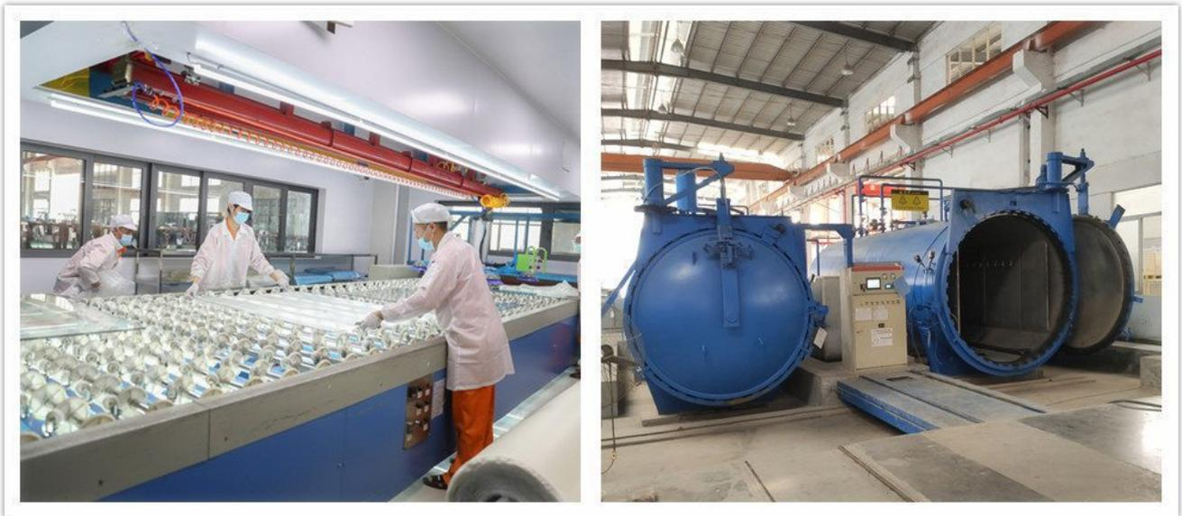
*dust-free lamination production and high temperature autoclave*
