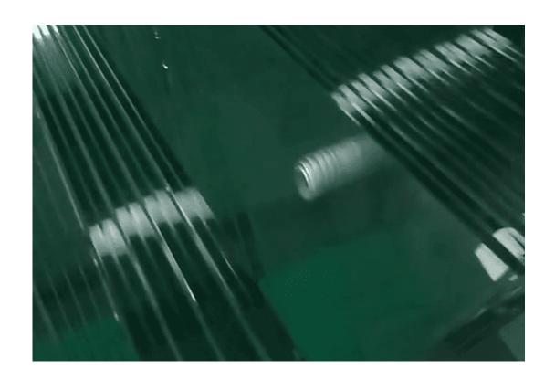
Laminated glass is made with two or more panes of glass that are held in place with the help of an interlayer to form a permanent and strong bond. The interlayer is typically made of Polyvinyl Butyral (PVB). The PVB interlayer bonds with both the layers of the glass and hold it together to form one strong, intact uniformed layer upon a harsh impact. This bond between the PVB sheet and the glass is a chemical bond and thus it does not shatter easily.
