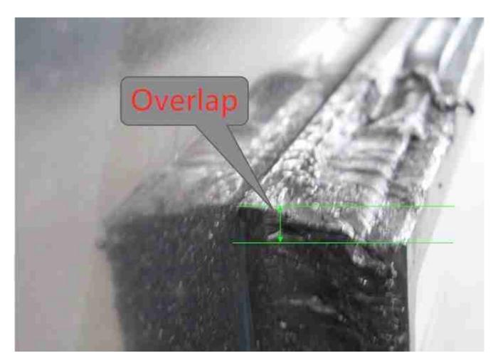
This looks familiar, right? Overlap is one of the most common flaws in DGU glass production. Especially when the quality controlling system is not strict enough, clients may receive production with this kind. Well, check the production which is made by our intelligent processing plant here:
