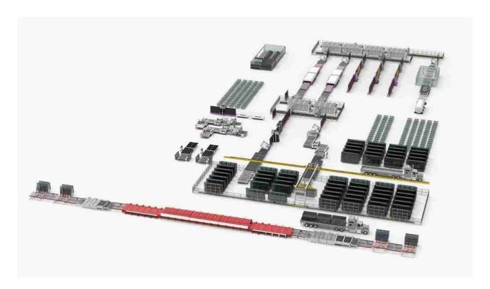
The image above is the brief view of our intelligent plant. It is built by the Lisec company from Austria. Total line needs about 10~15 human labours whereas the double insulating glass production(DGU) capacity reaches up to 60000SQM/month, this is 3~4 times comparing to the traditional plant.
