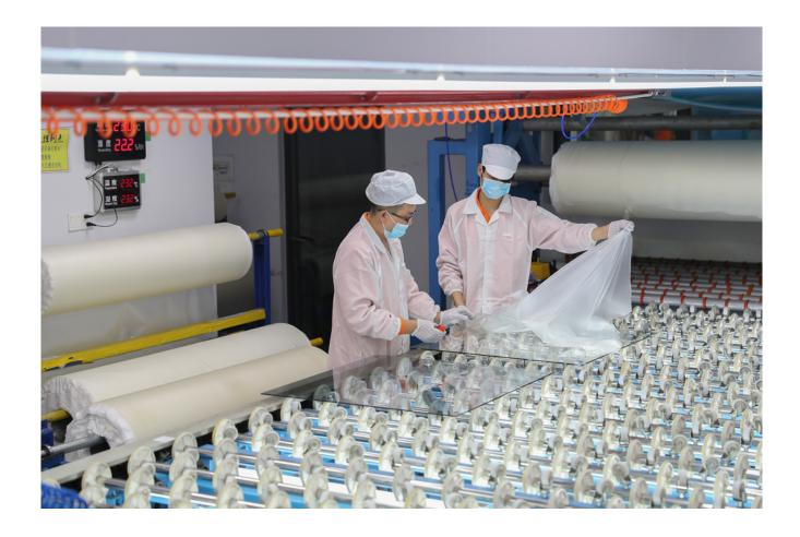
**Cutting:** Using high performance 6mm euro grey reflective glass and 6mm low-e glass, cutting to ultimate size according to drawings.
