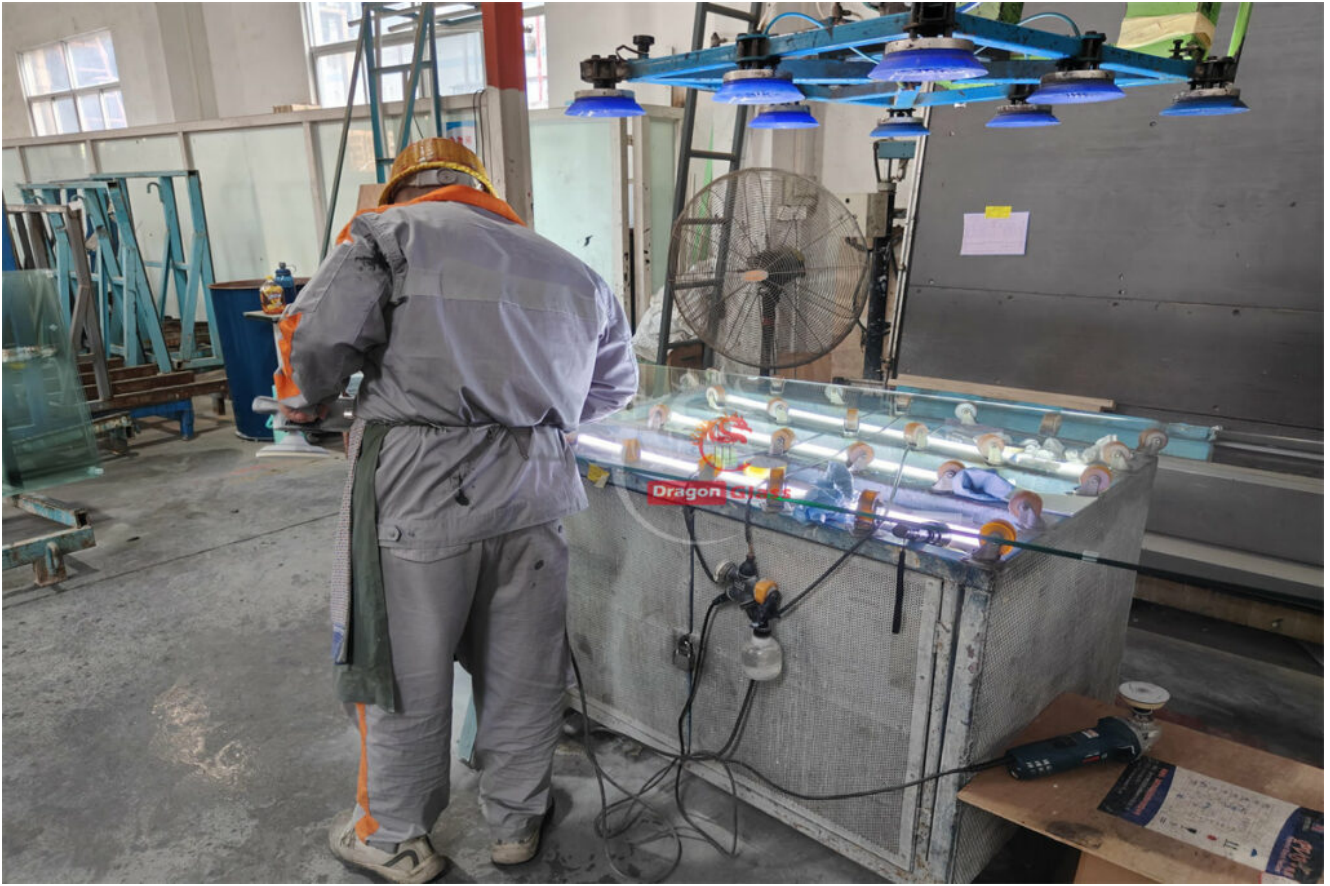
Laminated glass inspection by flashlight in Dragon Glass
