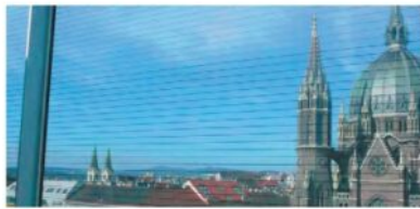
Horizontal black lines, 2 mm in diameter and with a 28 mm interval had very good Flight Tunnel test results
