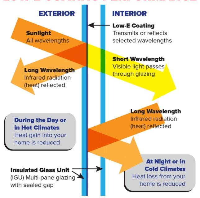
Low-E coatings have been developed to minimize the amount of ultraviolet and infrared light that can pass through glass without compromising the amount of visible light that is transmitted, is better able to retain heat during the winter and keep cool during the summer.
