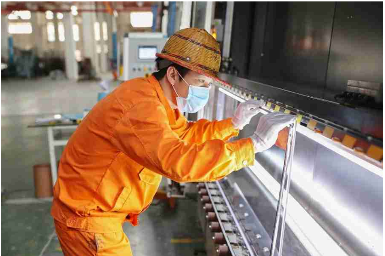
Carefully matching the size of spacer and the glass with the butyl sealant.
