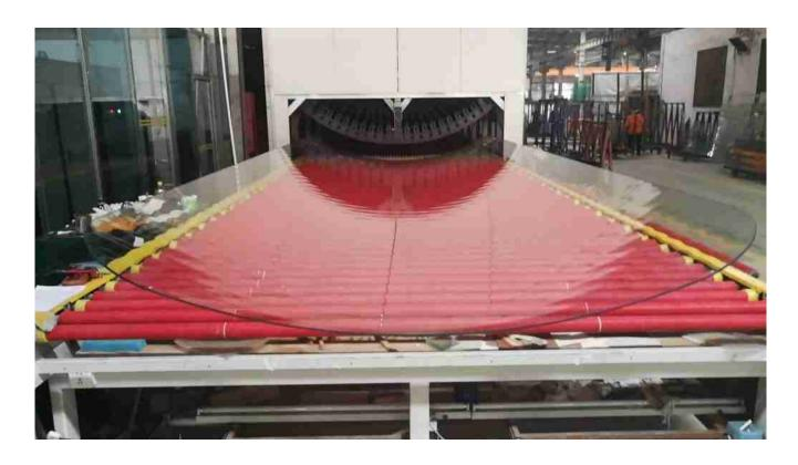
Curved tempering machine for producing curved glass
