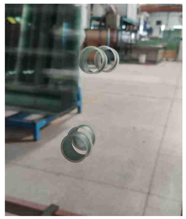
Drilling holes with accurate sizes and positions
