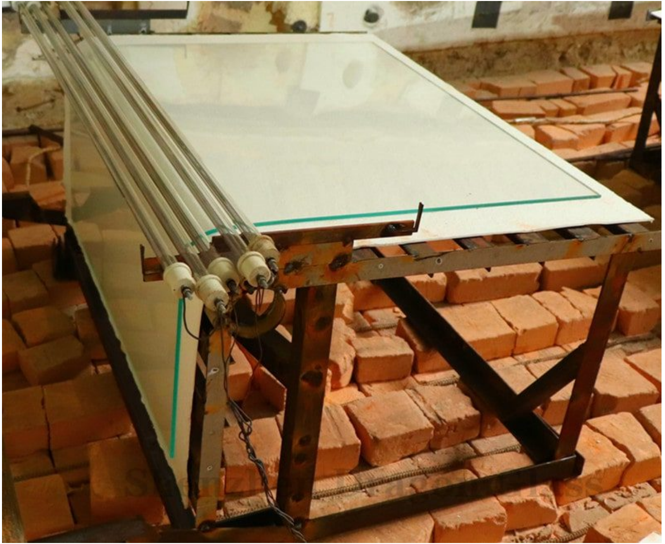
hot bending process
