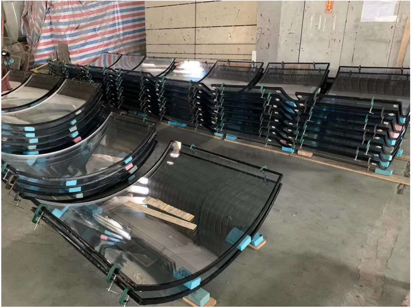
curved double glazed units for facade
