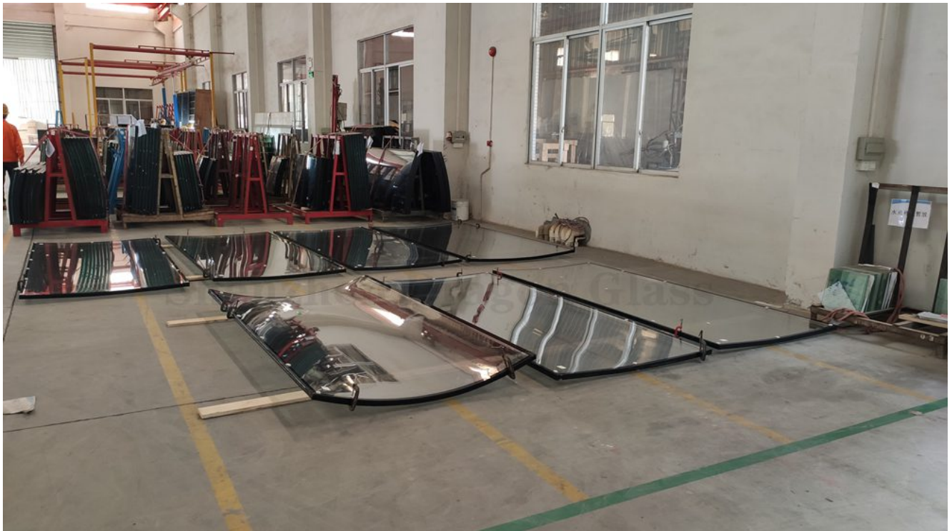
curved double glazed units for facade
