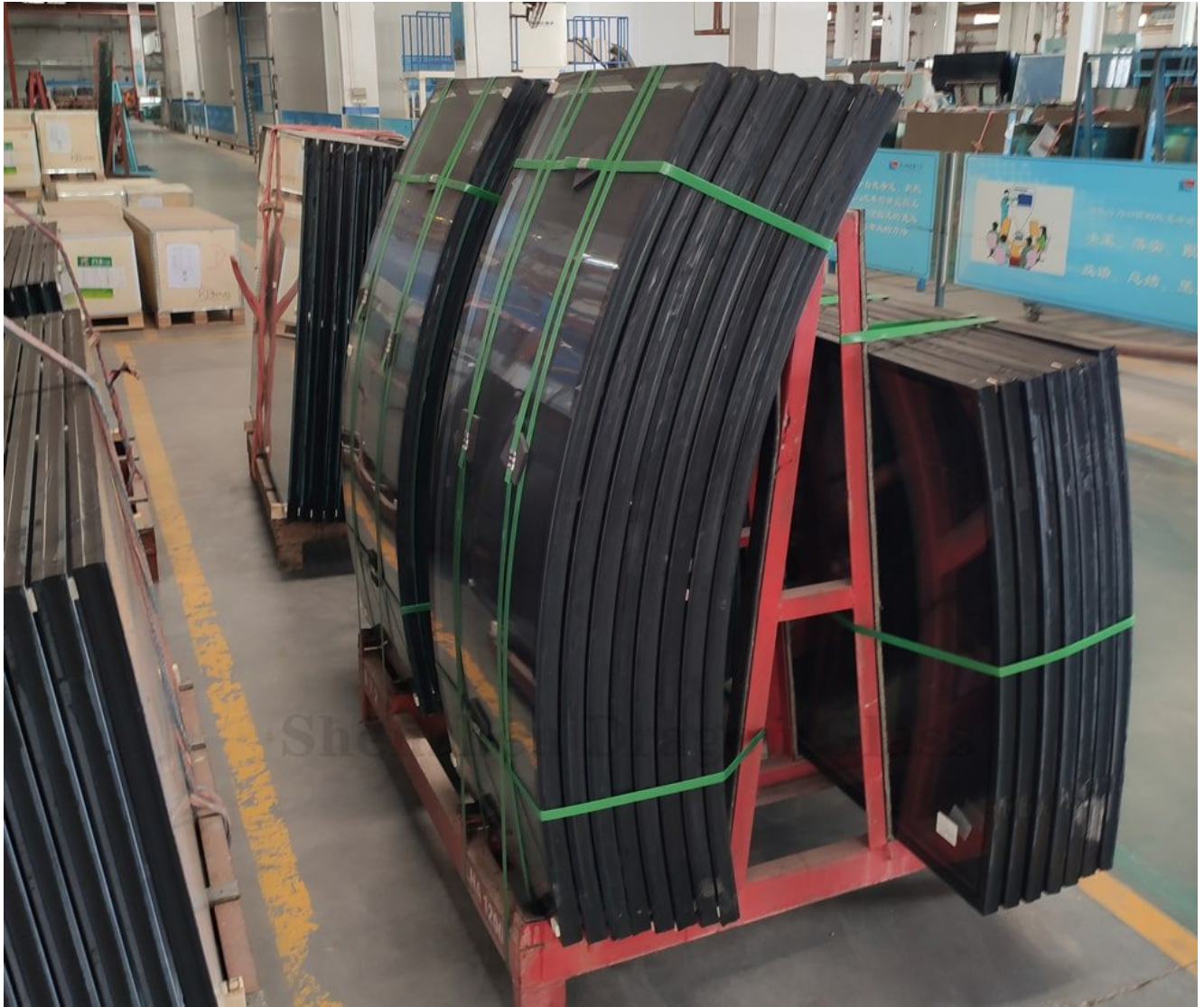
curved double glazed units for facade
