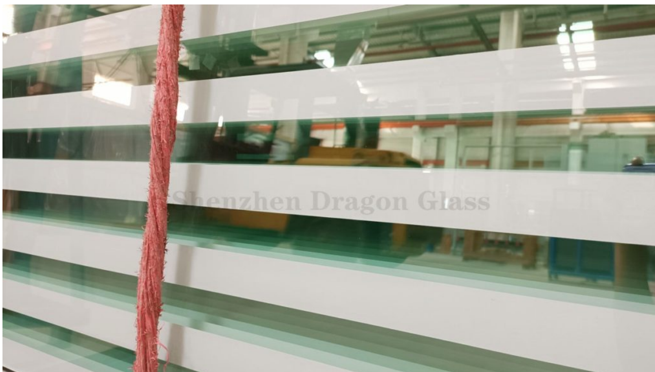
8mm+12A+8mm insulated glass panels for windows
