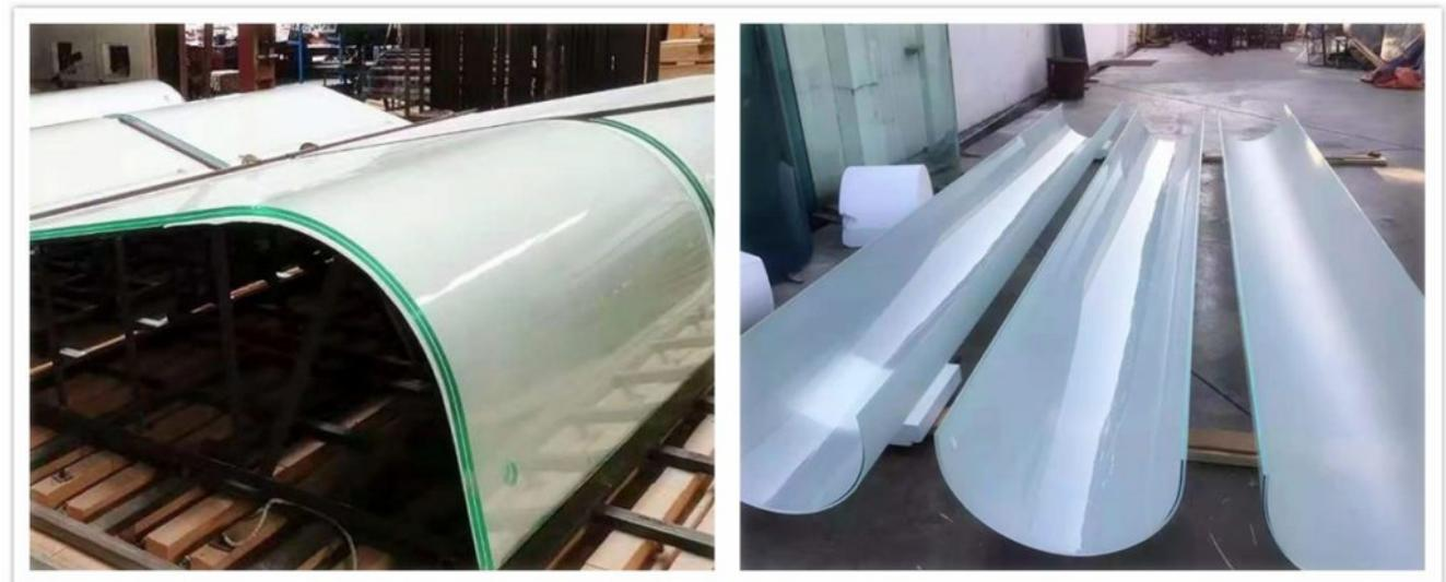
**Cold bending glass** is also called curved tempered glass, or curved toughened glass. It is processed in a tempering oven. After the desired shape is achieved in the curved mould in the tempering line. It will be cooled down rapidly to the room temperature with the strong windjet. Cold bending glass (curved toughened glass) has 5 times higher strength than normal annealed glass.
