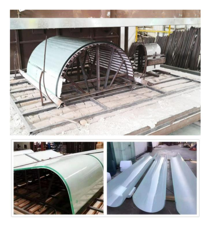
**Cold bending glass** is also called curved tempered glass, or curved toughened glass. It is processed in a tempering oven. After the desired shape is achieved in the curved mould in the tempering line. It will be cooled down rapidly to the room temperature with the strong windjet. Cold bending glass(curved toughened glass) has 5 times higher strength than normal annealed glass.
