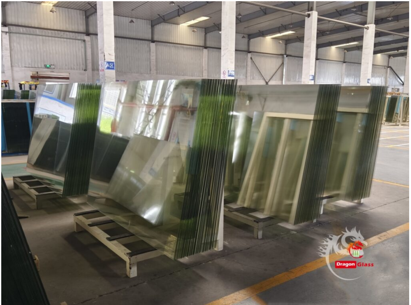
6mm borosilicate glass for fire door vision panel glass
