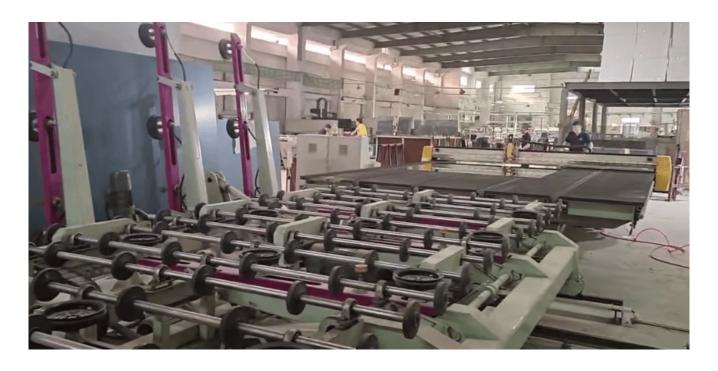
The auto cutting line as shown includes Equipment mainframe/equipment walking system/equipment transmission system/vacuum suction system / mechanical overturn the system.
