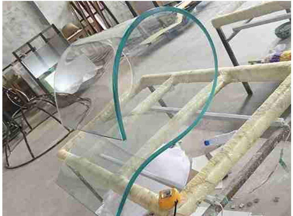
The original piece of glass is heated in a hot bending furnace to the glass softening point and later cools down slowly to room temperature. During the cooling process, it will form a specific shape according to the mold by its weight
