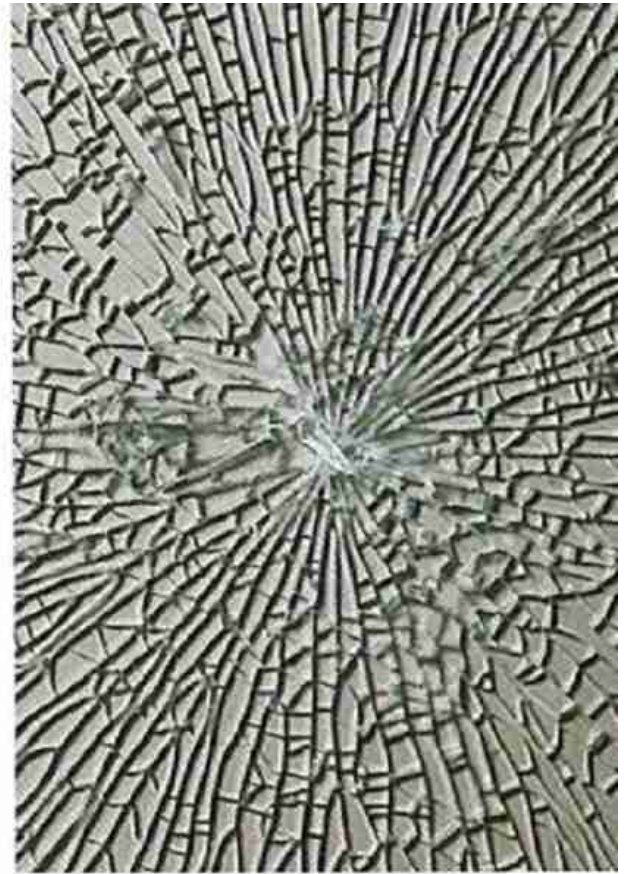
Breakage pattern – Tempered Glass
