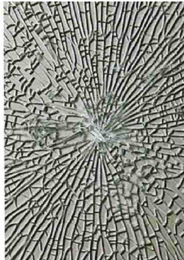
Breakage pattern – Tempered Glass
