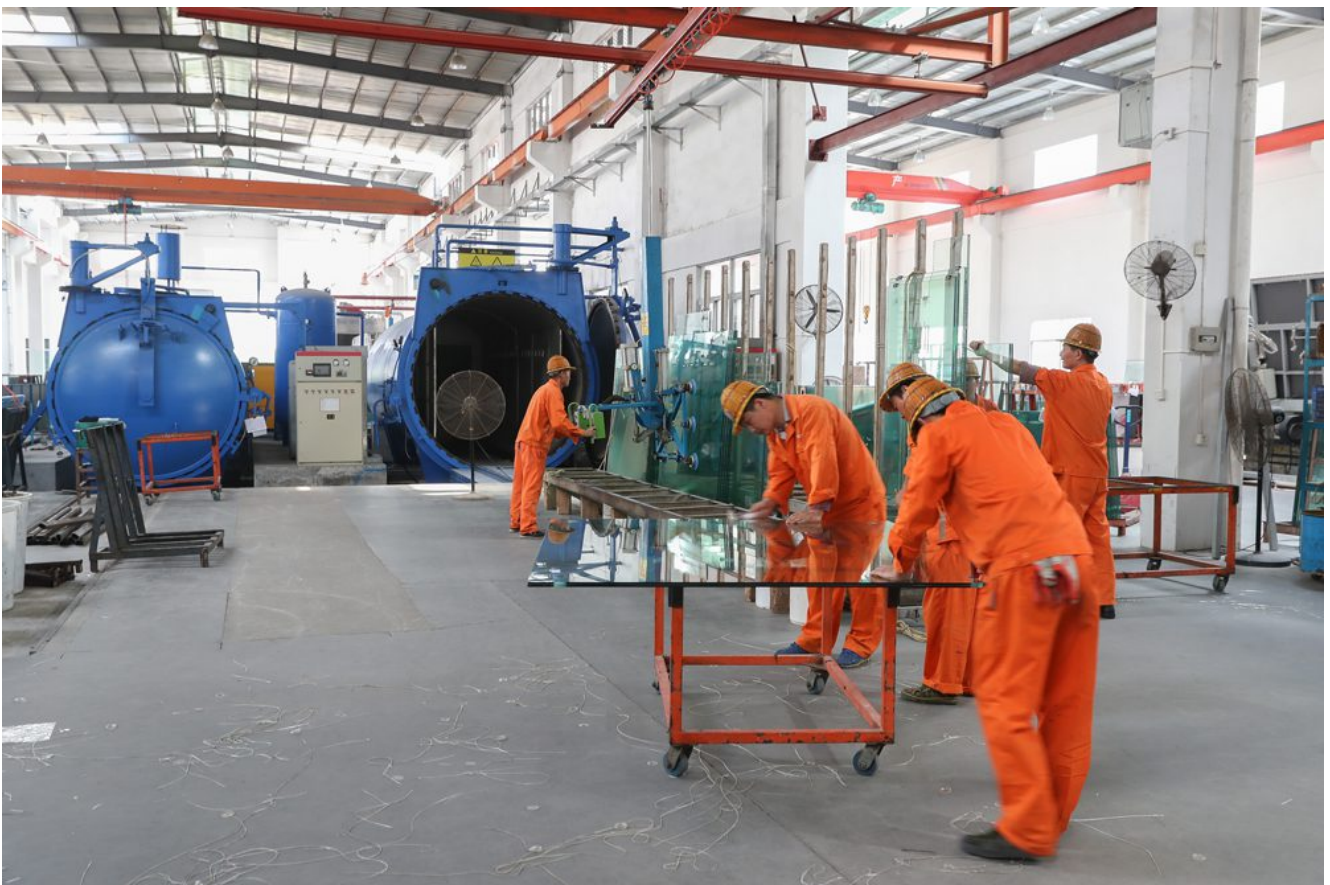
the remaining interlayers are being trimmed
