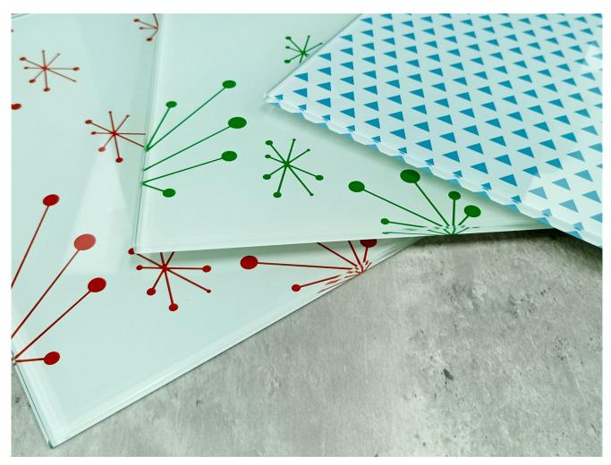
Silk screen printing glass also called <u>ceramic fritted glass</u>, is a type of decorative glass. The patterns are made by printing a layer of ceramic ink on the glass surface through a screen mesh.
